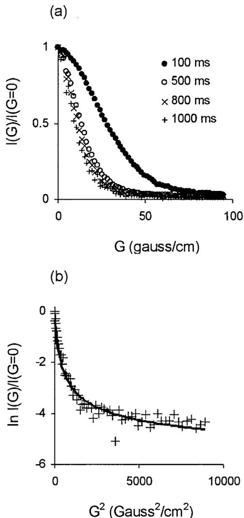
**Figure 8.** (a) Diffusion NMR data for a fabric sample made from AME(65) as a function of diffusion time. (b) Fit shown for a Gaussian distribution of pore sizes on the 1000 ms diffusion data. Average pore diameter was found to be 78  $\mu\text{m}$ .
