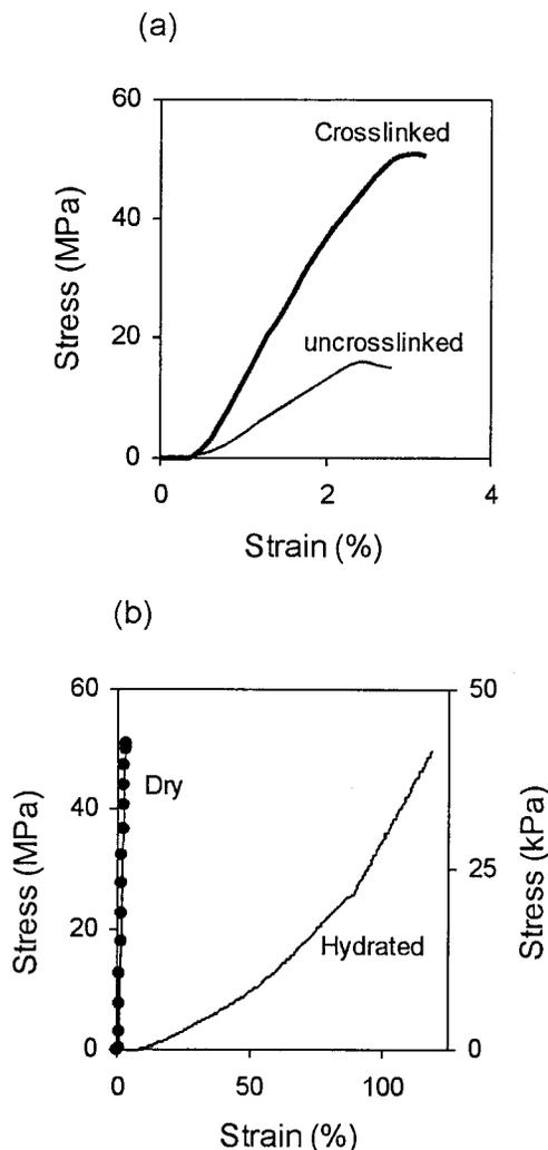
**Figure 9.** (a) Representative stress-strain curves of cross-linked and un-cross-linked fabric samples of AME(65) in the dry state. Cross-linking increases both tensile strength and modulus of the sample. (b) Representative stress-strain curves of dry ( $\bullet$ ) and hydrated cross-linked AME(65) fabric samples measured at a strain rate of 1  $\text{mm}/\text{min}$  at room temperature.
