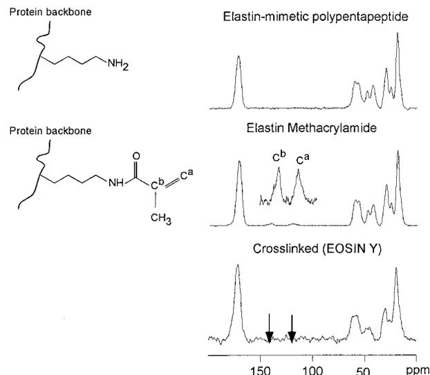
**Figure 4.**  $^{13}\text{C}$  CP/MAS/TOSS spectra of an elastin-mimetic protein polymer, methacrylate-modified elastin, and cross-linked elastin recorded at room temperature ( $23^\circ\text{C}$ ). Contact time = 1 ms and spinning speed ( $\omega_r/2\pi$ ) = 5 kHz. The disappearance of the peaks  $\text{C}^{\text{a}}$  and  $\text{C}^{\text{b}}$  in the spectrum for the cross-linked material indicates cross-linking after exposure to visible light.
