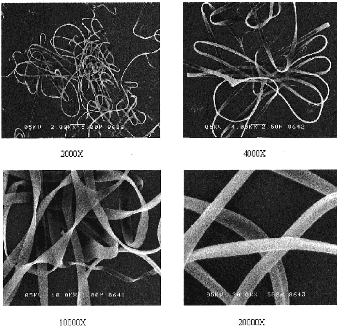
**Figure 6.** SEM micrographs of fibers spun from a 10 wt % AME(65) solution at room temperature. Flow rate = 50  $\mu\text{L}/\text{min}$ ; photoinitiator = EY (3 wt % of protein content). Long uniform fibers are produced with occasional triangle type bifurcation points. Fibers in the diameter range from 300 to 500 nm were produced.
