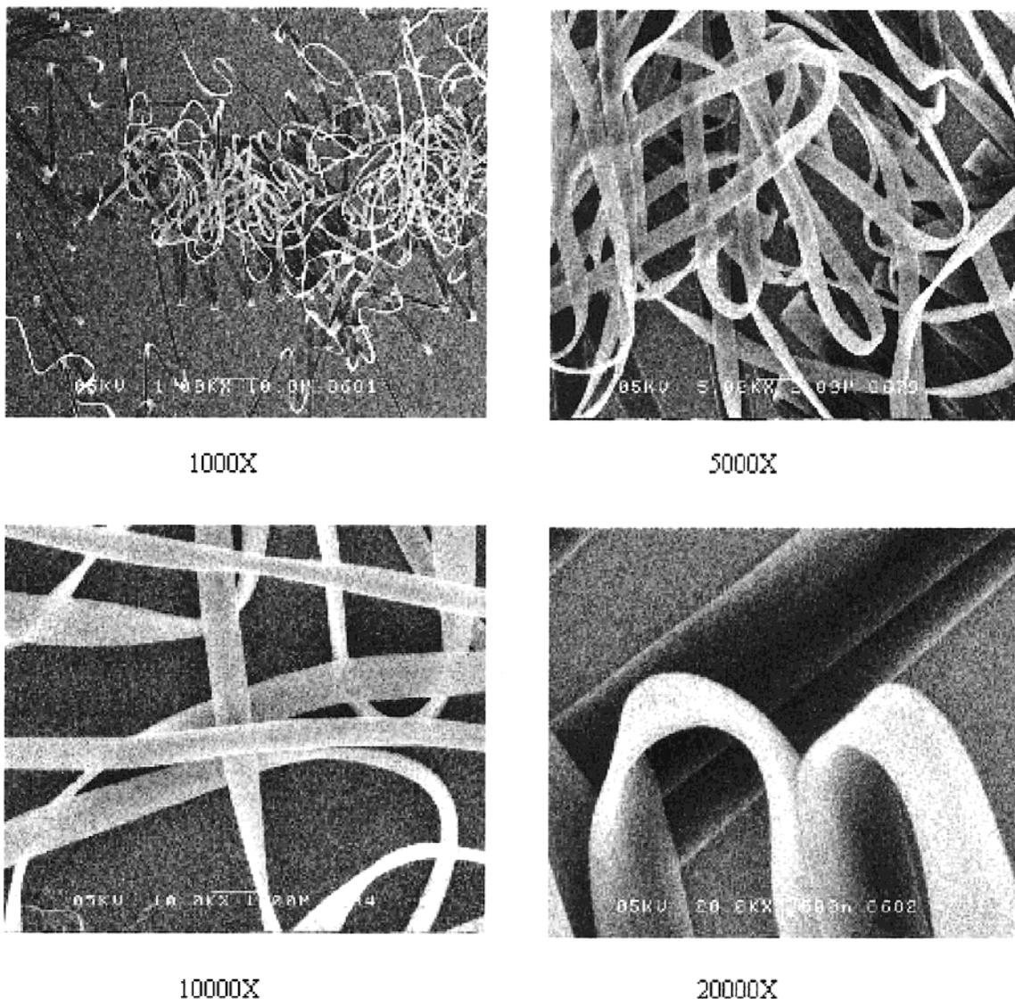
**Figure 7.** SEM micrographs of fibers spun from a 15 wt % AME(65) solution at room temperature. Flow rate = 50  $\mu\text{L}/\text{min}$ ; photoinitiator = EY (3 wt % of protein content). Long uniform fibers are produced with a flattened or ribbon-shaped morphology. Fibers in a variety of diameter ranges are produced (typically from 300 nm to 1.5  $\mu\text{m}$ ).
