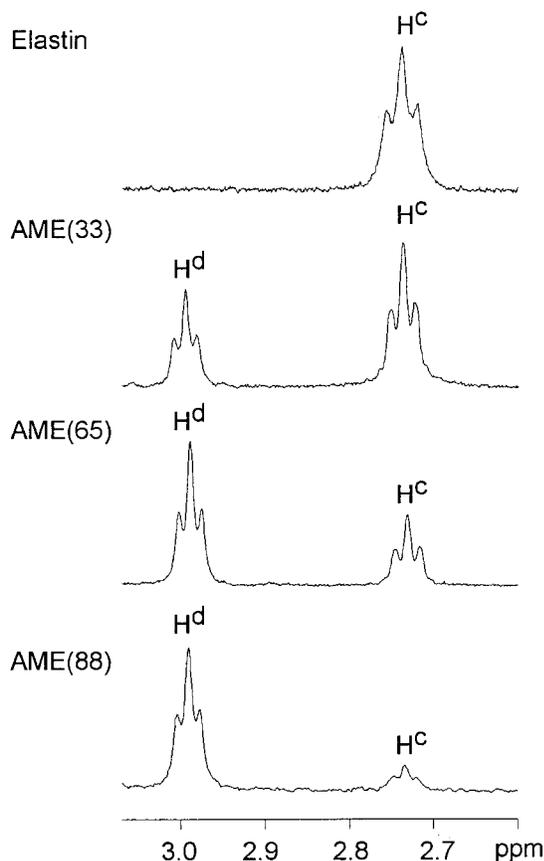
**Figure 2.**  $^1\text{H}$  NMR spectra of elastin and AME. The DOF of AME's is provided in parentheses. The expanded portion of the spectra between 2.6 and 3.1 ppm is shown. As DOF increases, the  $\text{H}^{\text{d}}$  peak grows in intensity at the expense of the  $\text{H}^{\text{c}}$  peak. The DOF can be computed from the integrated intensities of the  $\text{H}^{\text{c}}$  and  $\text{H}^{\text{d}}$  peaks.
