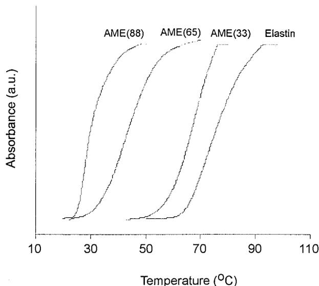
**Figure 3.** Temperature-dependent turbidimetry data for elastin and acrylate-modified elastin with different degrees of functionalization. The inverse transition temperature ( $T_i$ ) decreases with increase in the degree of functionalization (DOF). DOF dictates the temperature (processing window) at which fibers can be formed from aqueous solutions. The temperature window to the left of  $T_i$  is amenable for fiber formation.
