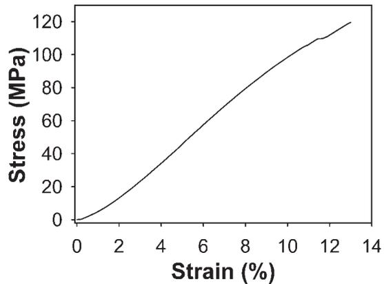
Figure 5. Representative stress-strain data for AC fiber.
