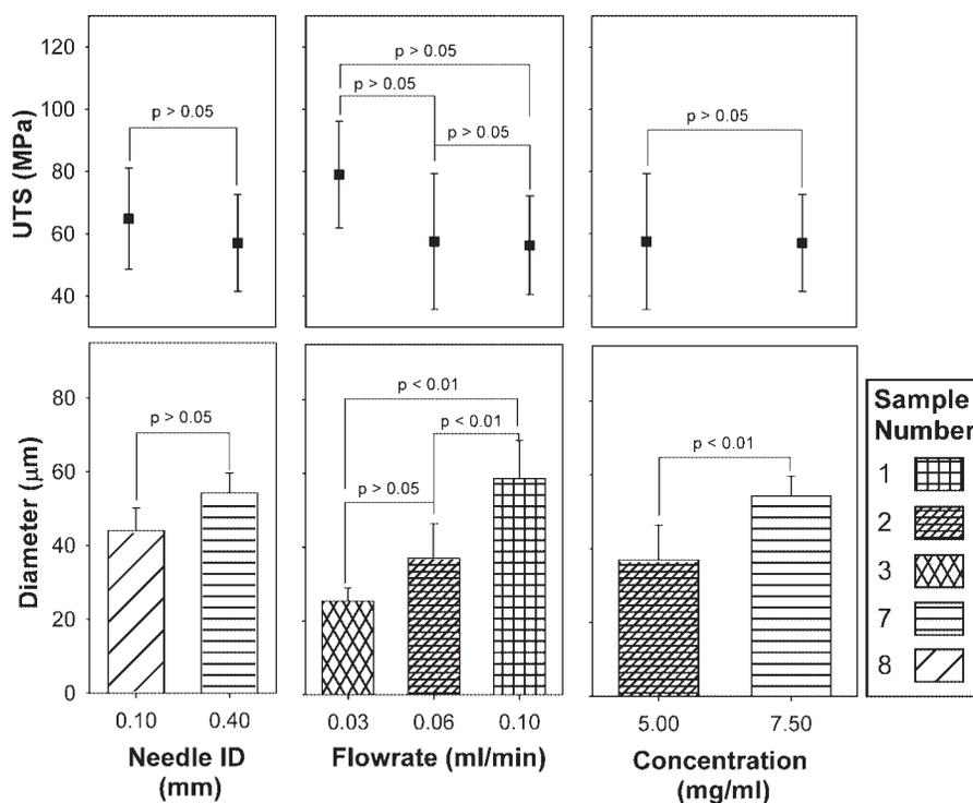
Figure 4. Mean UTS and major diameters of crosslinked MC fiber with varied wet spinning parameters. Sample numbers correspond to the parameters in Table I. Error bars represent standard deviations.
