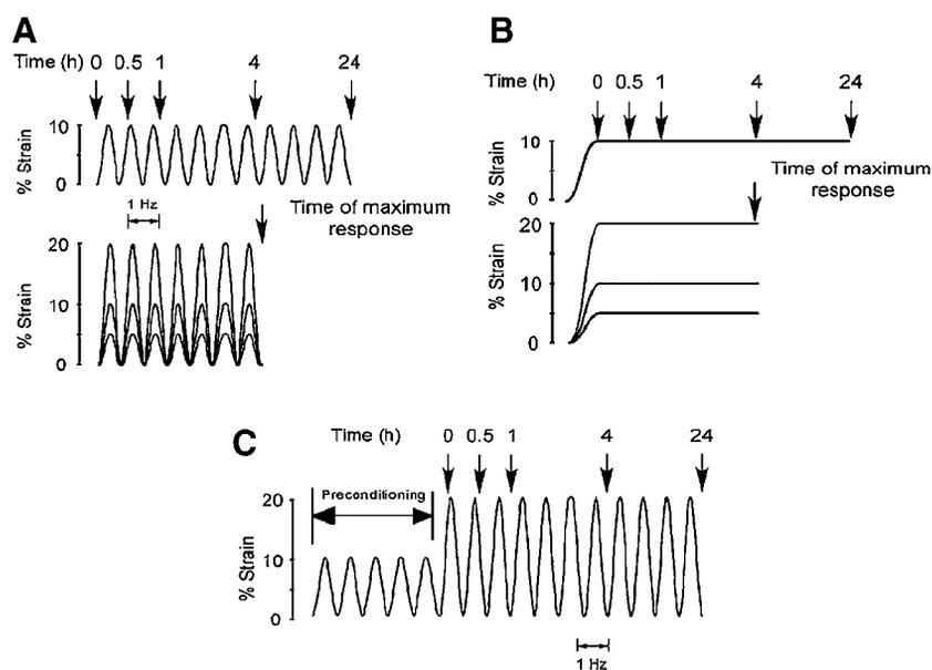
**Fig. 1.** Protocols for the application of mechanical strain. SMCs were subjected to 1 Hz cyclic tension for various time periods and strain magnitudes (A). Alternatively, cells were subjected to static tension (B). The effect of preconditioning was examined by cyclically stretching the cells at 10% strain for 24 h, followed by 20% cyclic strain (C). Arrows indicate sampling points, in which cells were harvested for analysis.
